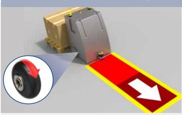
Incremental encoders inputs can be directly read by LASER SENTINEL in order to select the appropriate slow-down and stopping areas, depending on the speed of the vehicle
