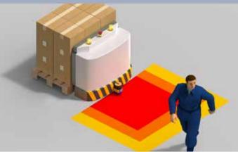
Warning and Safe areas can be used to warn operators, slow down the vehicle or stop it only when needed. Up to 70 different area sets can be configured and activated depending on position, speed and movement of vehicle.
