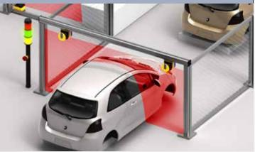
LASER SENTINEL is the only system that thanks to its master/ slave architecture can manage combined applications where multiple zones stop different parts of the machine, without any need of external controller.
