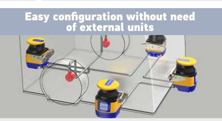
Up to 4 LASER SENTINEL can be easily connected to each other through Ethernet-based safe communication bus. Only one of them, the Master, receives power, has inputs and outputs onboard and keeps the memory of the configuration of the entire system. The other scanners, the Slaves, are connected to the Master with a single cable that also give them power.
