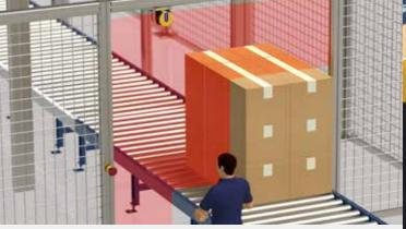
LASER SENTINEL can be configured to mute an area of variable size and position, depending on the working phase of the machine. Muting activation is done by muting sensors activated by the approaching of the load that has to enter or exit the dangerous area. Override function is also available in order to restart the movement after an unintended stop.
